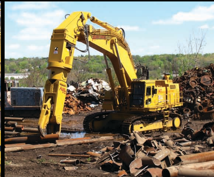
Well drill pipe processed with the Allied-Gator MT™ Series Multi-Tool
