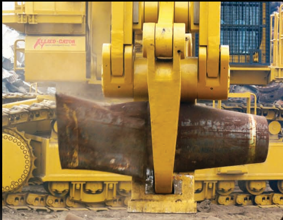
Well drill pipe processed with the Allied-Gator MT™ Series Multi-Tool
